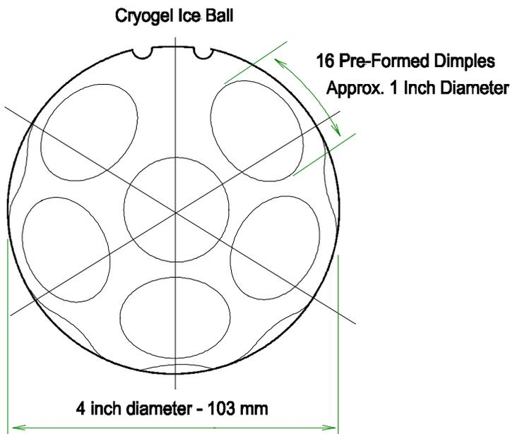
Ice Balls are constructed with a proprietary high performance polyethylene polymer. HDPE
