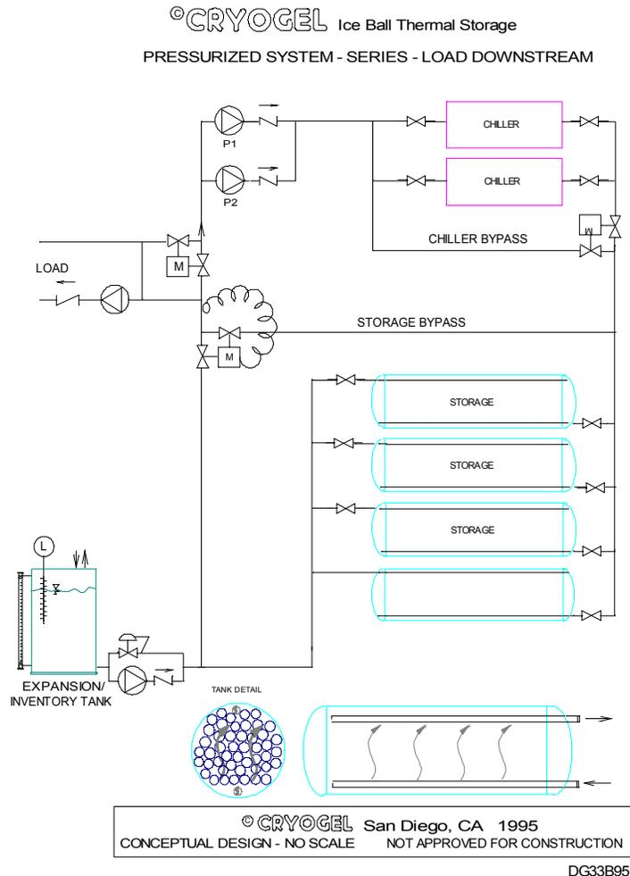
As the water freezes inside the Ice Balls and as the Ice Ball dimples flex outward, glycol solution surrounding the balls is displaced. This fluid displacement can be monitored to provide information as to the amount of ice in storage at any time. (See Ice Inventory Control.)
