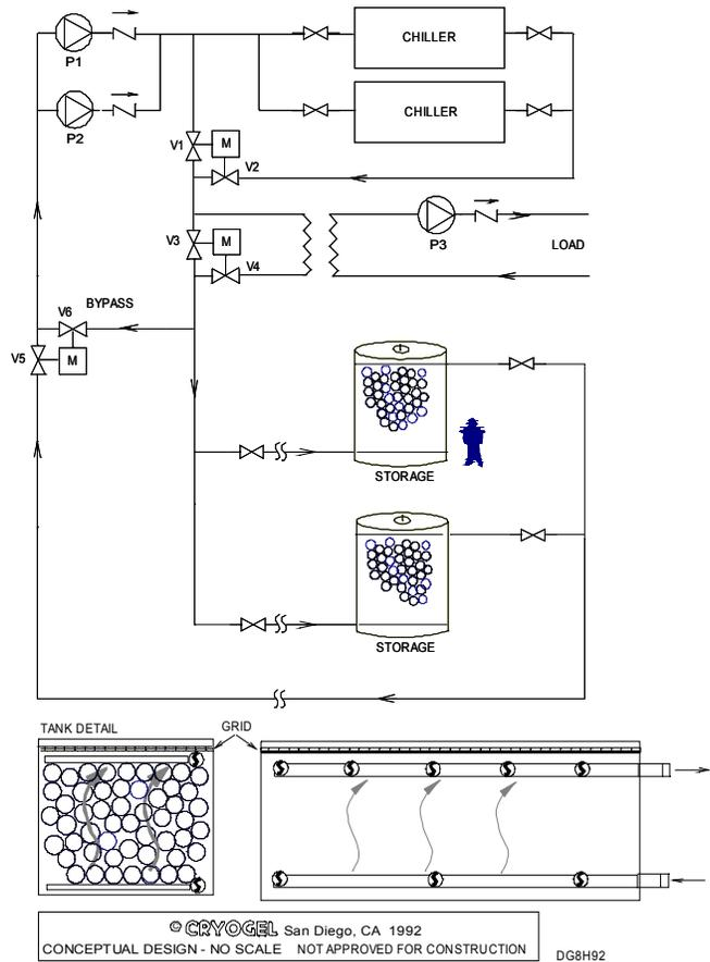
Since ice floats inside the ball during the melt mode, and since the balls are flexible, the ice remains in contact with the interior wall of each Ice Ball, which improves heat transfer between the ice and the glycol solution. While it may go without saying, the Ice Balls move only slightly due to flexure of the dimples during freezing and melting... the Ice Balls do not move around within the tank or piping.
