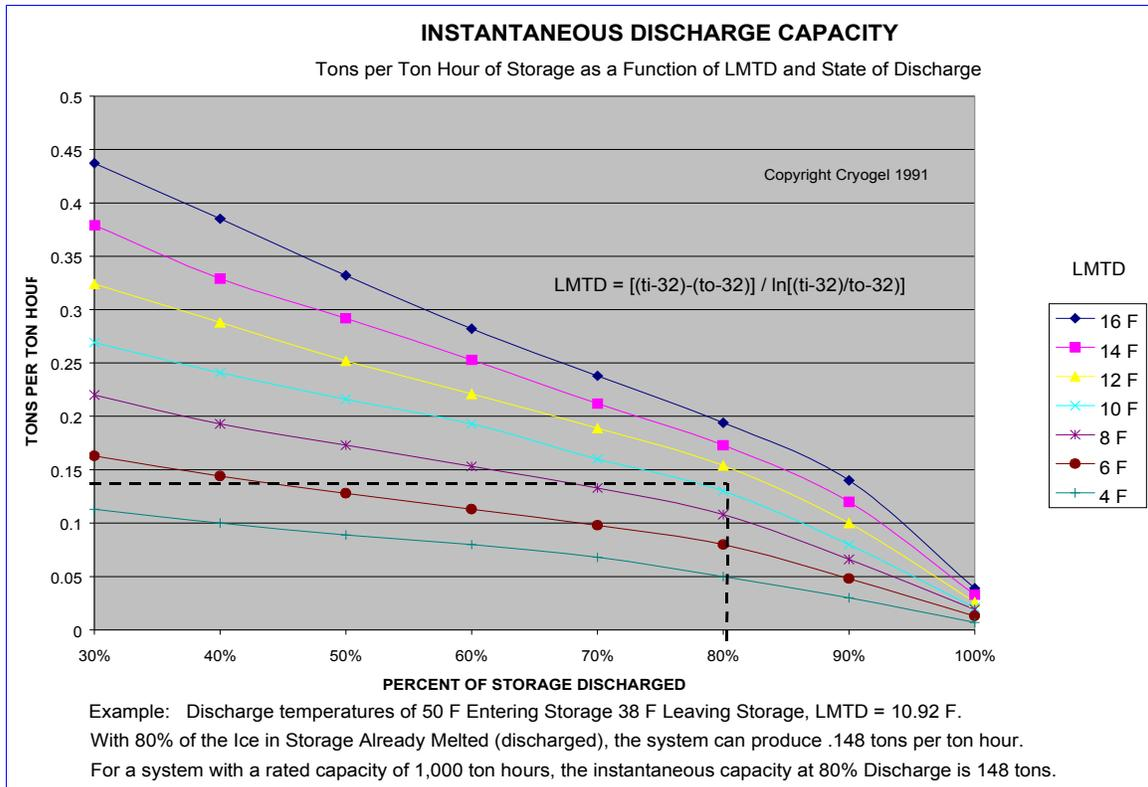
Cryogel sizing is based on independent laboratory test data. Cryogel has assembled that data into a set of performance curves. These curves represent the ability of the Ice Balls to transfer heat based upon the percentage of ice in the tanks and the Log Mean Temperature Differential (LMTD) across the tanks. This is similar to the methodology heat exchanger manufacturers use for sizing of their equipment.
